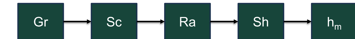
Figure 3. Process of calculating the convective mass transfer coefficient (variables are Grashof, Schmidt, Rayleigh, and Sherwood respectively)
